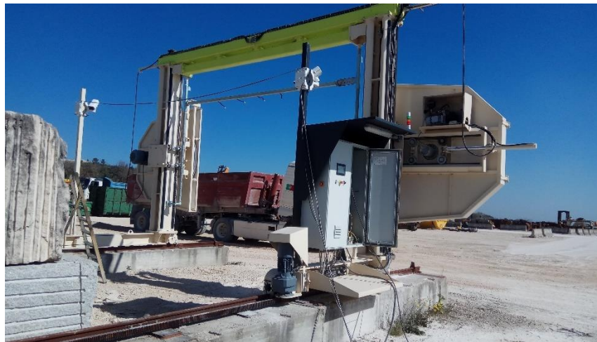
Figure 3: Camera set up in a Limestone quarry
