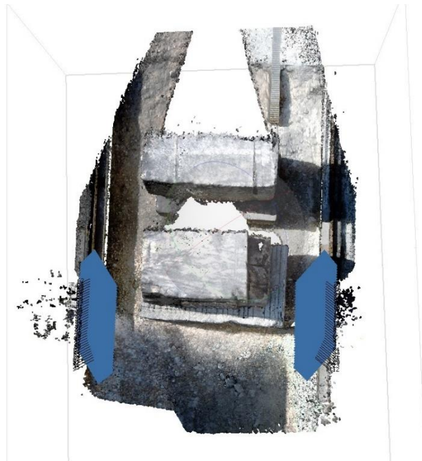
Figure 53: Top view of dense point cloud from Agisoft Metashape
